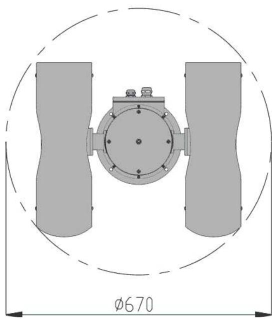
**SCHEMA DI FORATURA PER FISSAGGIO PTX200**
